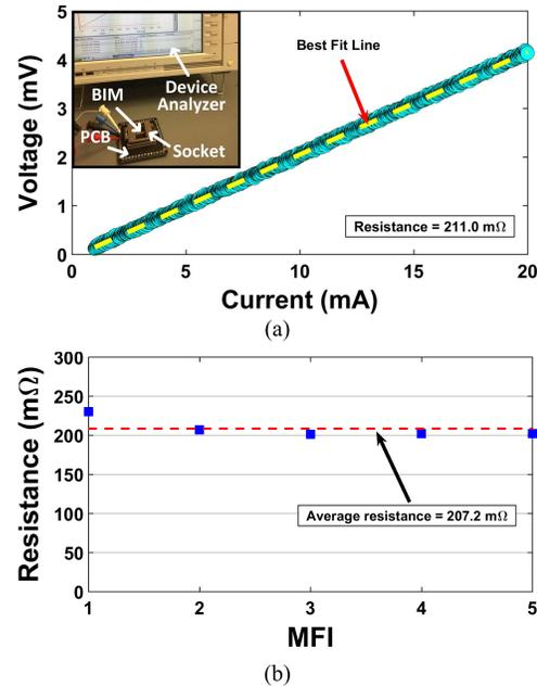
Fig. 4. (a) Four-point resistance setup and extracted resistance from an IV curve of one of the MFIs on the BIM and (b) four-point resistance measurements (including contact resistance) for five different MFIs ( $2.1 \mu\text{m}$  thick) on the same BIM sample.
