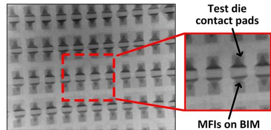
Fig. 3. X-ray image showing alignment between MFIs and corresponding electrodes on the test die.
