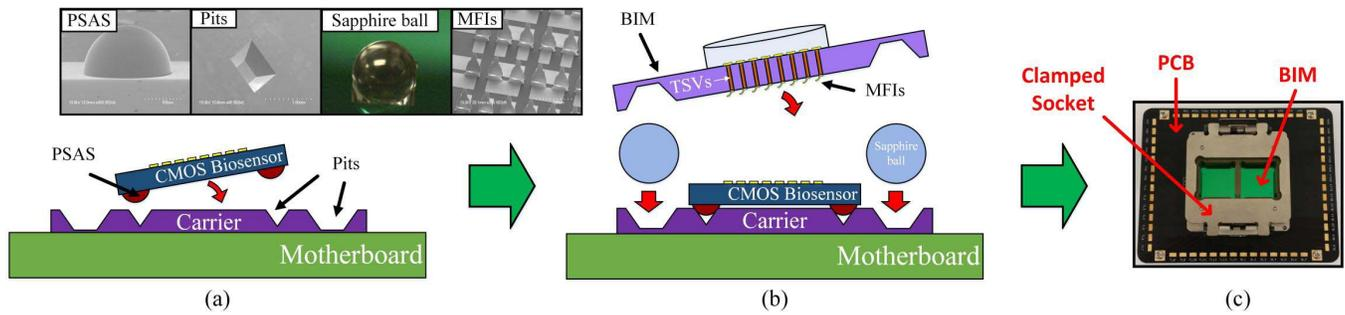
Fig. 2. Double self-alignment process flow demonstrating two levels of self-alignment: (a) CMOS biosensor to carrier self-alignment via a PSAS/pit mechanism, (b) BIM to carrier self-alignment via a sapphire ball/pit mechanism. Final clamped state (c) follows.
