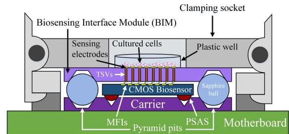
Fig. 1. Biosensing-interface module (BIM) in modular system.
