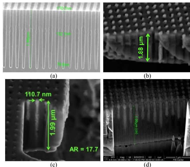
Fig. 9. Fabricated nanoscale TSVs (a) blind  $\sim 100$  nm diameter vias, (b) and (c) cross section of fully plated TSVs, and (d) cross section with copper removed near via bottom during focused ion beam (FIB) cross sectioning
