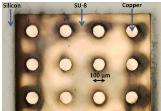
Fig. 3. Top view of the fabricated polymer-embedded vias
