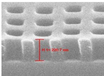
Fig. 8. Cross section of 100 nm diameter openings in developed photoresist
