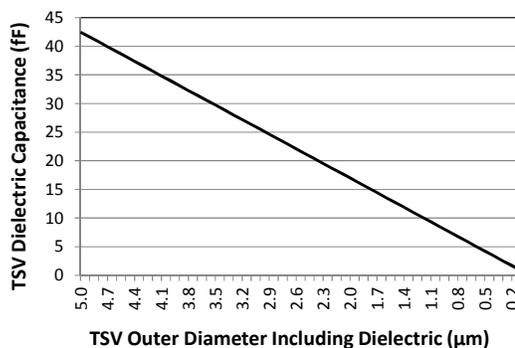
Fig. 6. TSV dielectric capacitance as a function of TSV outer diameter
