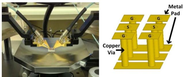
Fig. 4. RF probe setup (left) and GSG TSV structure for simulations and measurements of polymer-embedded vias (right)
