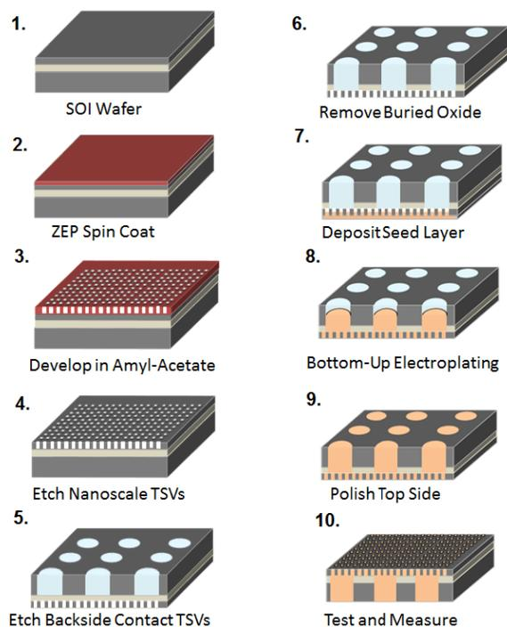
Fig. 7. Fabrication process for nanoscale TSVs
