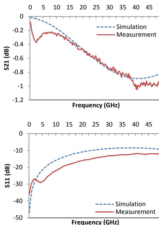
Fig. 5. High-frequency simulation and measurement results for polymer-embedded vias with via-trace-via structure
