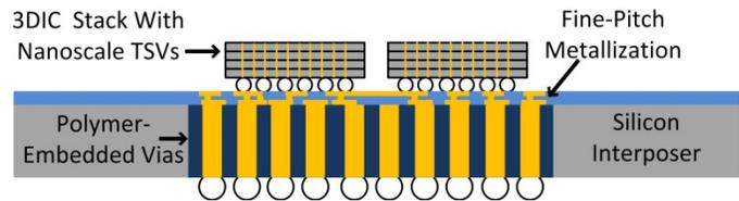
Fig. 1. Silicon interposer with polymer-embedded vias and 3D ICs consisting of ultra-dense nanoscale TSVs mounted atop the interposer
