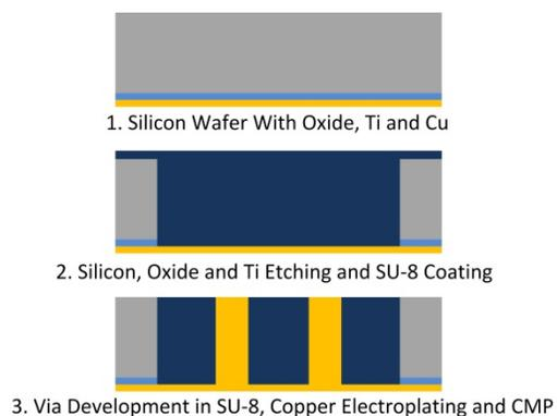
Fig. 2. Fabrication process for polymer-embedded vias
