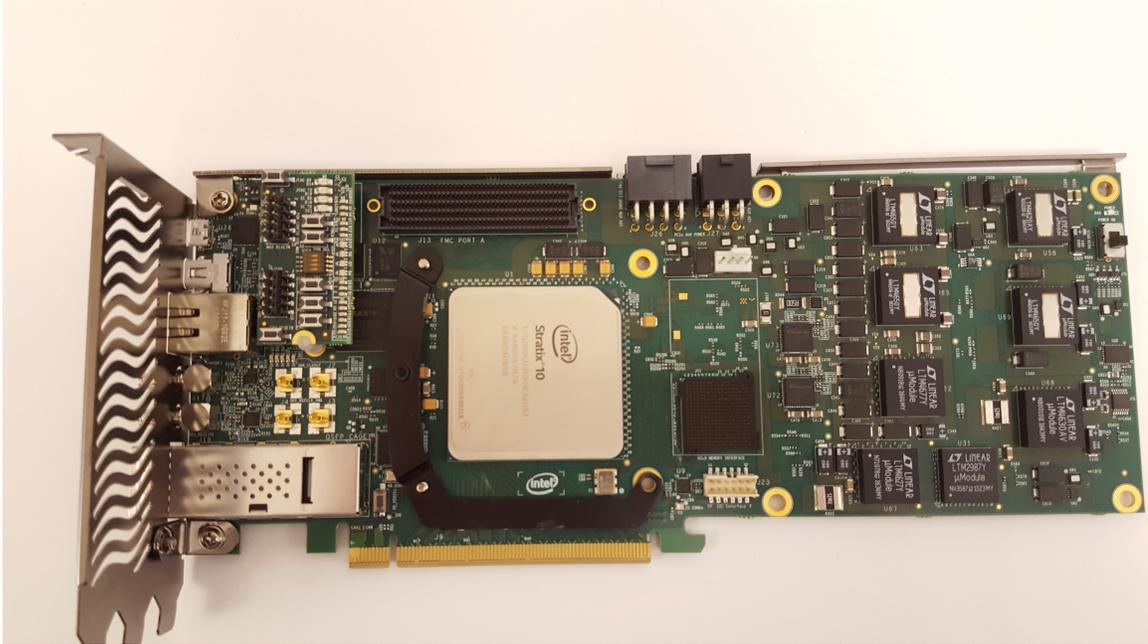
Figure 4.5: Intel Stratix 10 ES development kit with the Stratix 10 GX FPGA package attached.
