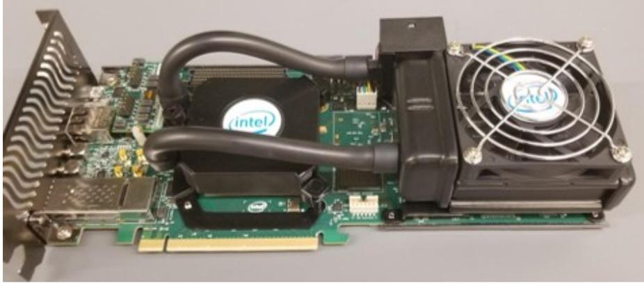
Figure 4.11: FPGA development board with stock heatsink.
