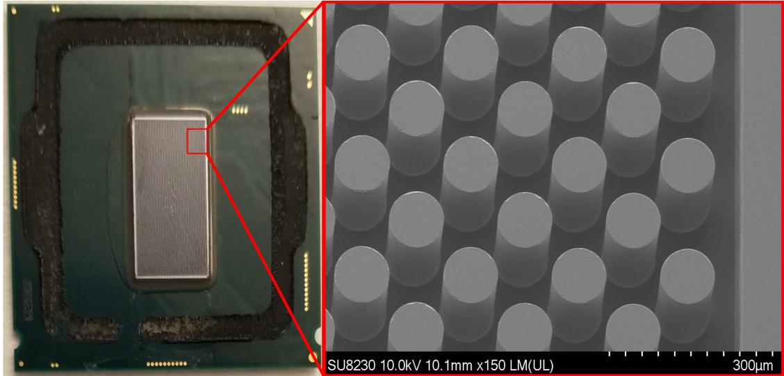
Figure 3.7: Photograph of the etched package with the insert showing an SEM of the micropin-fins.
