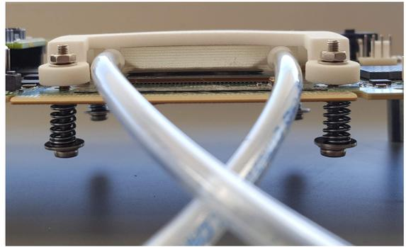
(b) Screws and springs applying pressure
