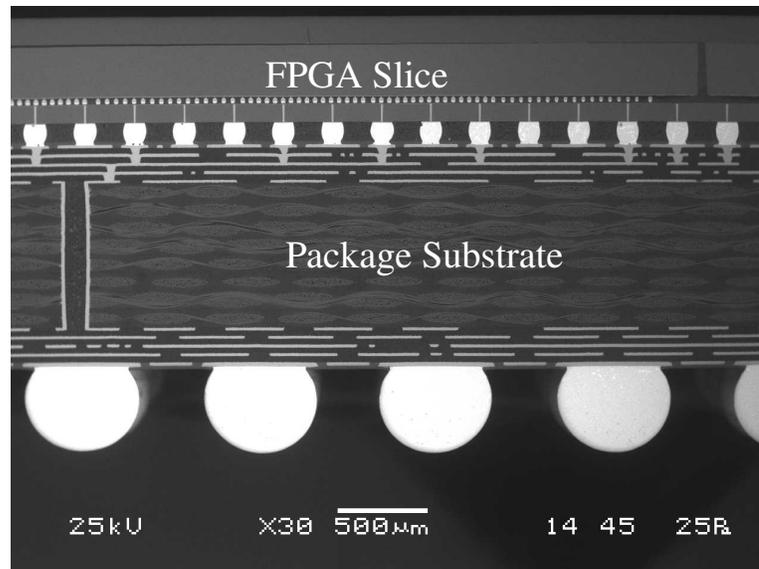
Figure 1.3: Cross section of Xilinx 28 nm FPGA on Interposer © 2012 IEEE [11]
