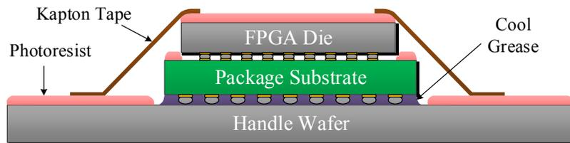
3) Etch Micropin-fins and remove handle wafer.
