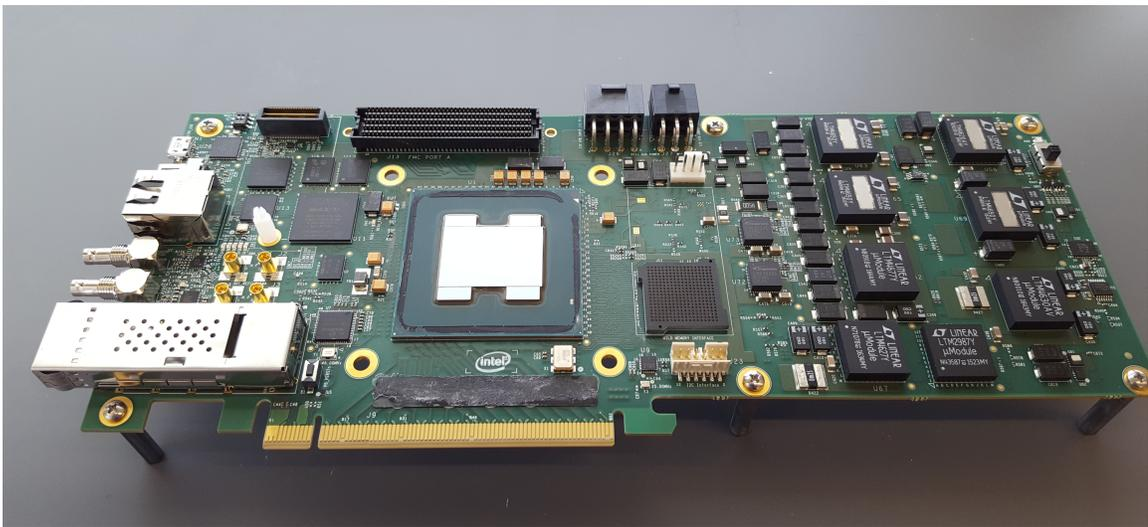
Figure 5.16: Delidded Stratix 10 FPGA on development board
