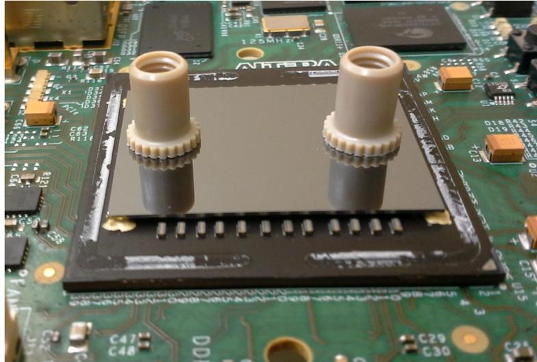
Figure 4.6: Processed FPGA soldered to development board with silicon cap and Nanoports for fluid delivery
