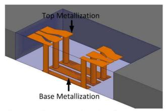
**Schematic of Structure for D-band Measurements**
