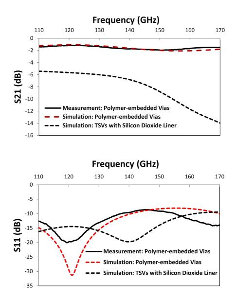
Figure 64: D-band measurements and simulations of a polymer-embedded via link; TSVs with silicon dioxide liner included for benchmarking.
