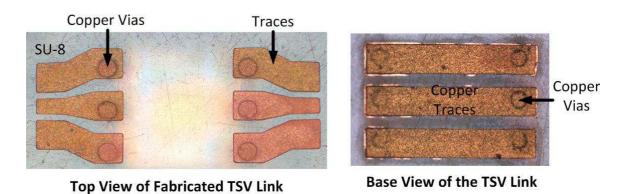
Figure 63: Fabricated polymer-embedded vias for measurements in the D band including traces with fan-in at top.
