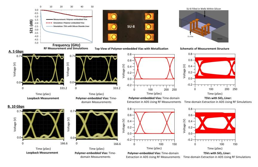
Figure 61: Measured eye diagrams of polymer-embedded vias (Figure 54) with constructed eye diagrams in ADS using the RF measurements of polymer-embedded via chains. Loopback measurement and extracted eye diagrams from the RF simulations of the TSVs with silicon dioxide liner are also shown for benchmarking.
