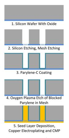
Figure 13: Fabrication process of parylene-clad TSVs.
