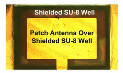
Figure 73: Fabricated patch antenna over a metal-coated polymer well.
