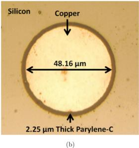
Figure 14: Parylene-clad TSV processing results (a) after mesh fabrication and Parylene-C deposition (left) and after oxygen plasma etch of Parylene blocking (right), and (b) after CMP showing the top view of the fabricated 390  $\mu$ m tall Parylene-clad TSVs with  $\sim\!48~\mu$ m diameter copper vias surrounded by a  $\sim\!2.25~\mu$ m thick cladding.
