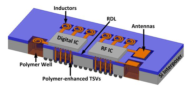
Figure 65: Envisioned mixed-signal silicon interposer platform featuring polymerenhanced TSVs, antennas and inductors.
