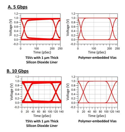
Figure 47: Eye diagrams of TSVs with silicon dioxide liner and polymer-embedded vias.
