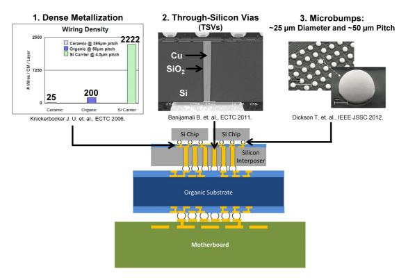
Figure 5: Schematic of a 2.5D system using silicon interposer technology with key components shown [24, 25, 29].
