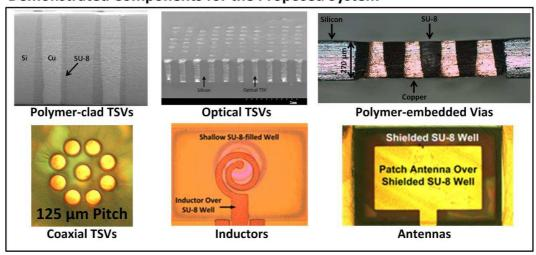
Figure 78: Proposed RF/mixed-signal large-scale interposer-based system with the key components demonstrated in this research for the system.
