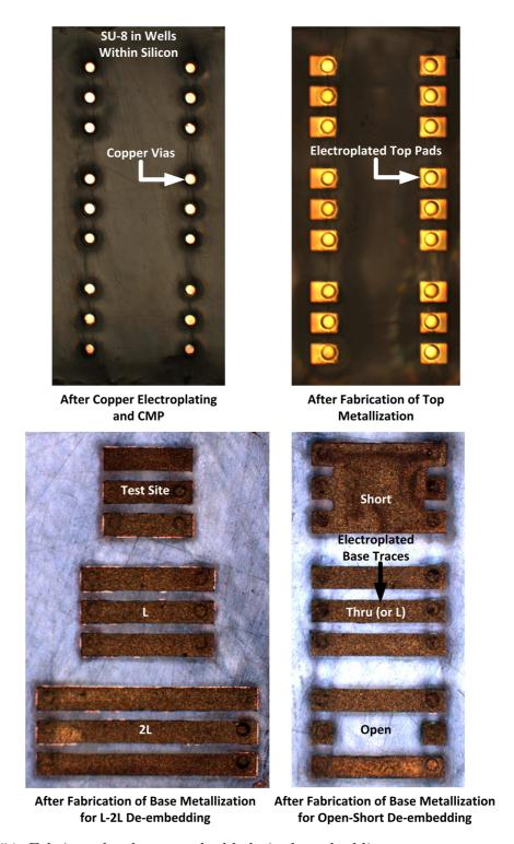
Figure 54: Fabricated polymer-embedded via de-embedding measurement structures.
