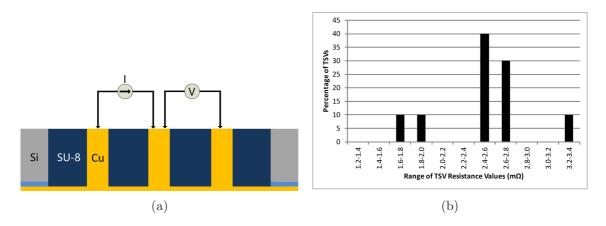
Figure 41: Resistance measurements of polymer-embedded vias with 100  $\mu$ m diameter and 270  $\mu$ m height: (a) Schematic of 4-point resistance measurement setup and (b) Distribution of 4-point resistance measurements for 20 polymer-embedded vias.
