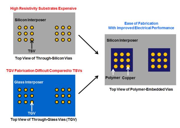
Figure 33: Comparison between through-silicon vias, through-glass vias and polymer-embedded vias.
