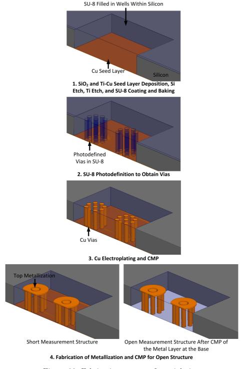
Figure 66: Fabrication process of coaxial vias.
