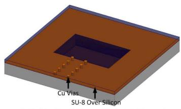
2. SU-8 Coating, Baking and Photodefinition, and Cu Electroplating and CMP
