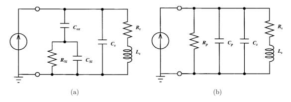
Figure 4: Inductor physical models: (a) Lumped model and (b) Equivalent circuit model using the lumped model [15].
