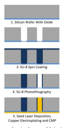
Figure 18: Fabrication process for simultaneous fabrication of photodefined optical and polymer-clad TSVs.
