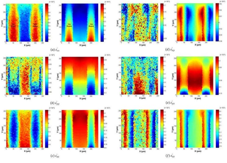
Figure 26: Measured deviatoric strain distribution maps of silicon (left) vs. model predicted strain maps (right) at 150 °C for the fabricated 50  $\mu$ m diameter and 300  $\mu$ m tall TSVs with 1  $\mu$ m thick silicon dioxide liner and on a 150  $\mu$ m pitch.
