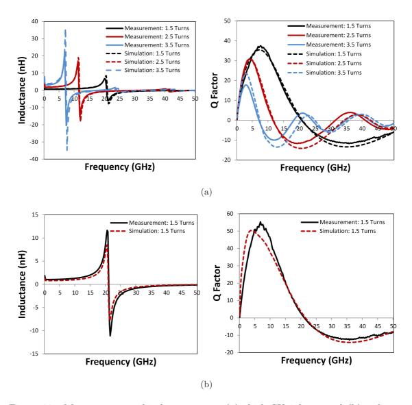
Figure 77: Measurements of inductors over: (a) thick SU-8 layer and (b) polymer well.
