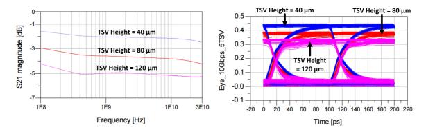
Figure 8: Impact of TSV length on insertion loss and eye diagram [36].
