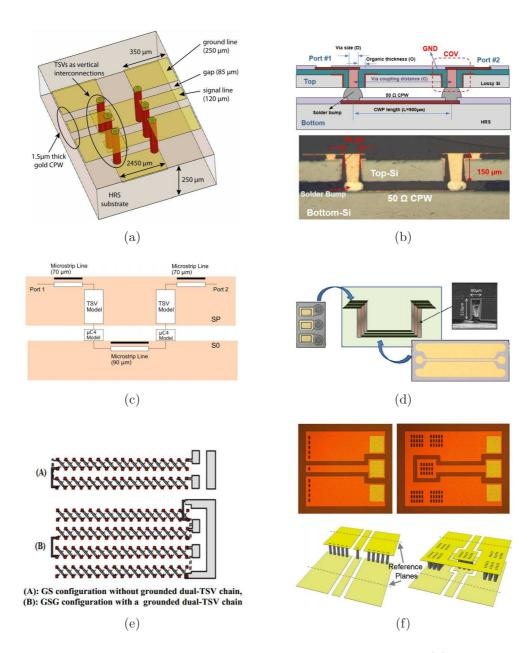
Figure 48: TSV RF measurement structures in the literature for: (a) TSVs with gold coated nickel wires assembled magnetically [106]; (b) coaxial structures with laser ablated polymer-filled vias [84]; (c) TSV loss characterization in CMOS SOI technology [104]; (d) characterization of TSVs in high-resistivity silicon for RF interposer applications [107]; (e) characterization of tungsten-filled dual-TSV chains [102]; and (f) implementation of TRL de-embedding using TSV bundles [108].
