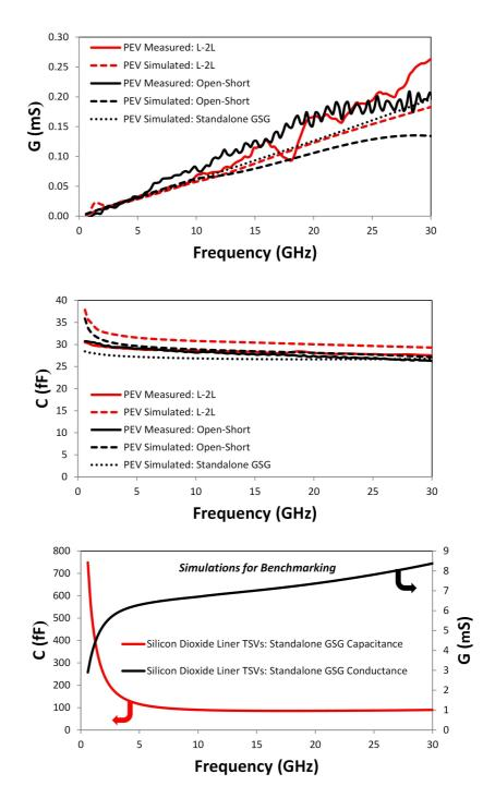
Figure 56: Extracted conductance and capacitance of the de-embedded polymer-embedded vias (PEVs) using measurements and simulations; TSVs with silicon dioxide liner included for benchmarking.
