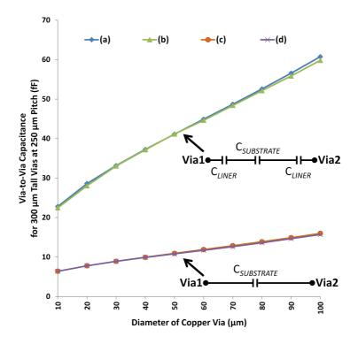
Figure 34: Via-to-via capacitance for passive silicon interposers: (a) Using the model for TSVs with a 1 m thick silicon dioxide liner; (b) Using Raphael simulations for TSVs with a 1  $\mu$ m thick silicon dioxide liner; (c) Using the model for polymerembedded vias; and (d) Using Raphael simulations for polymer-embedded vias.
