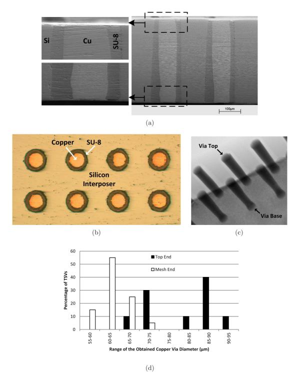
Figure 17: Fabricated 390  $\mu$ m tall SU-8-clad TSVs with  $\sim$ 80  $\mu$ m diameter copper vias surrounded by a  $\sim$ 20  $\mu$ m thick cladding on a 250  $\mu$ m pitch: (a) Cross section view; (b) Top view; (c) X-ray image showing void-free copper electroplating; and (d) Distribution of the obtained copper via diameters of 20 measured polymer-clad TSVs.
