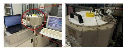
Figure 30: OES setup with sensor mounted on top of ICP etching tool process chamber (closer image shown on the right).
