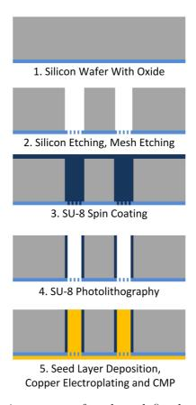
Figure 15: Fabrication process for photodefined polymer-clad TSVs.
