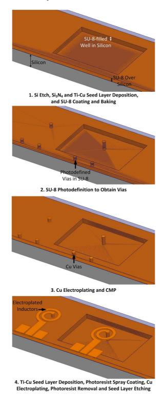
Figure 75: Fabrication process of polymer-enhanced inductors.
