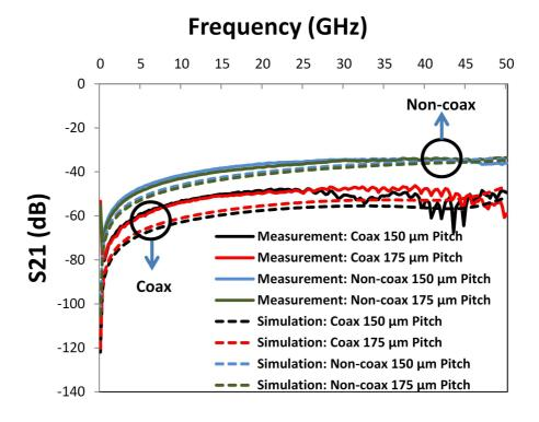
Figure 71: Coupling measurements of the fabricated polymer-enhanced coaxial and non-coaxial TSVs.
