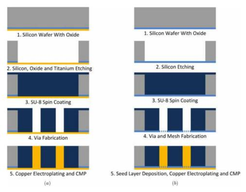
Figure 35: Fabrication processes for polymer-embedded vias: (a) Process with copper support layer and (b) Process with mesh seed layer.
