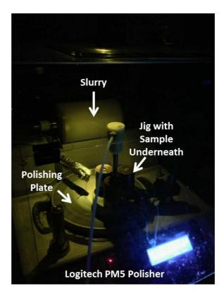
Figure 36: An image of the setup used to polish uncrosslinked SU-8 in an ultra-low light environment.
