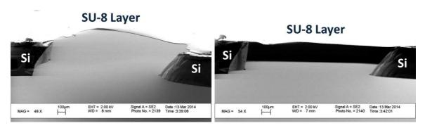
Figure 80: Fabricated suspended SU-8 wells.
