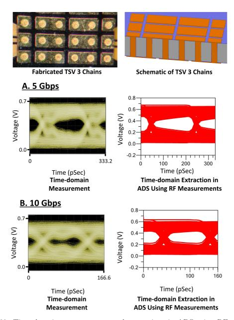
Figure 60: Time-domain measurements and extractions in ADS using RF measurements for TSV 3 chains.
