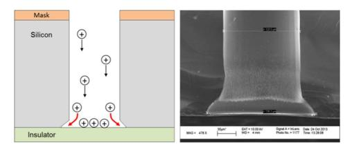
Figure 28: Notching mechanism in TSV fabrication using BOSCH process (Left) and cross-section of a 120  $\mu$ m diameter via showing notching at the base (Right).
