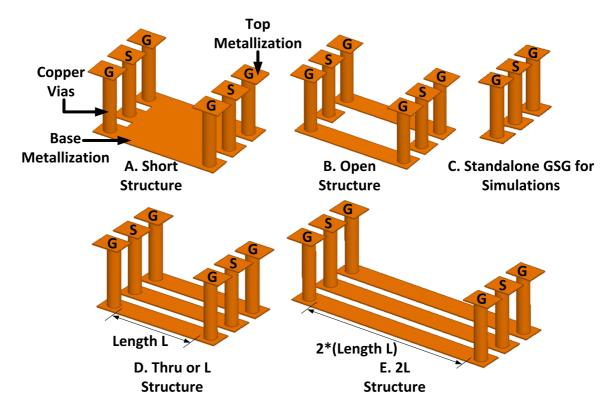
Figure 53: Schematic of measured and simulated TSV structures for de-embedding.
