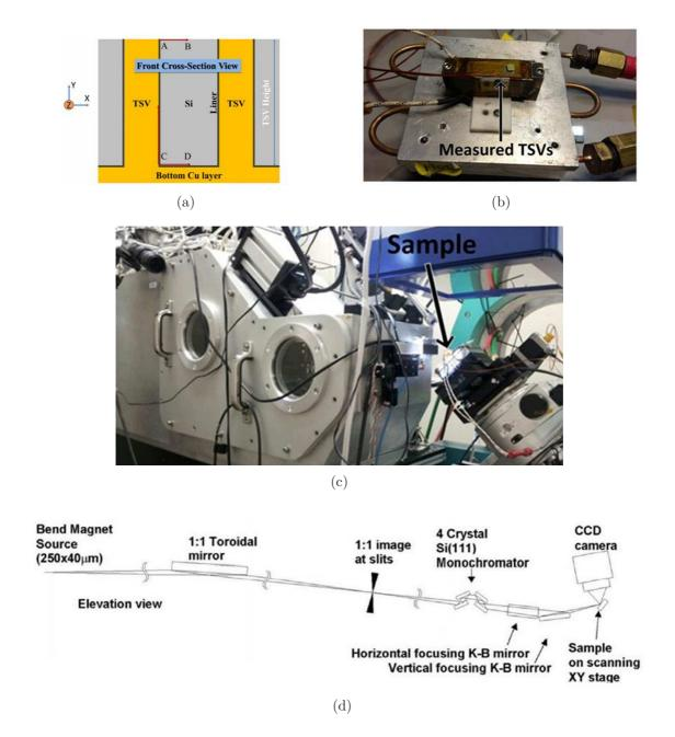
Figure 24: Synchrotron XRD setup for TSV strain measurements: (a) Schematic of the TSV area measured; (b) Setup of a TSV sample attached to a heater; (c) Beamline setup with the TSV sample; and (d) Schematic layout of the beamline [74].
