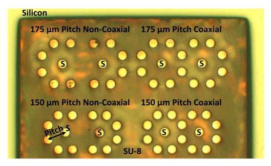
Figure 70: Fabricated polymer-enhanced coaxial vias and non-coaxial vias (for benchmarking).
