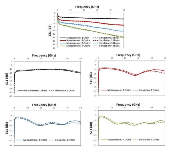
Figure 52: RF measurements and simulations of TSVs with silicon dioxide liner.
