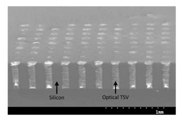
Figure 19: Fabricated 390  $\mu$ m tall optical TSVs with a 118  $\mu$ m diameter SU-8 core surrounded by a 2  $\mu$ m thick silicon dioxide cladding on a 250  $\mu$ m pitch.
