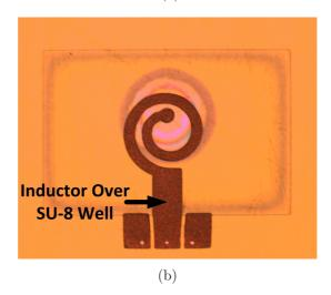
Figure 76: Fabricated inductors over: (a) thick SU-8 layer and (b) polymer well.
