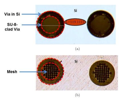
Figure 16: Fabricated 390  $\mu$ m tall SU-8-clad vias with  $\sim$ 80  $\mu$ m diameter openings and  $\sim$ 20  $\mu$ m thick cladding on a 250  $\mu$ m pitch: (a) Top view and (b) Base view.
