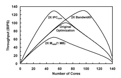
Figure 2: Plot showing performance improvement in a many-core chip with high memory bandwidth [9].
