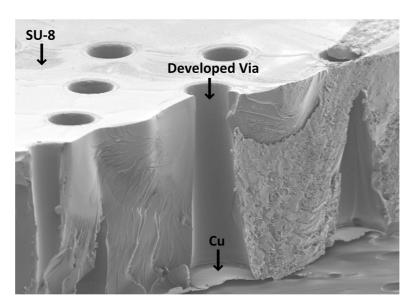
Figure 37: Cross section of a polymer-embedded via after SU-8 development.
