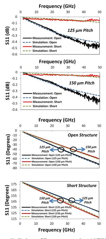
Figure 68: Single-port RF measurements of coaxial TSVs.
