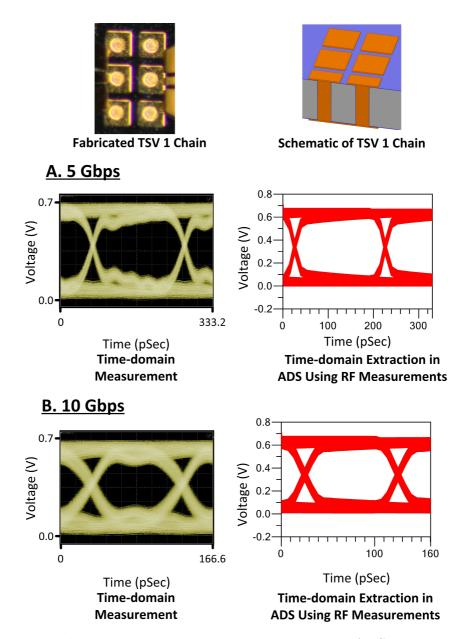
Figure 59: Time-domain measurements and extractions in ADS using RF measurements for TSV 1 chain.
