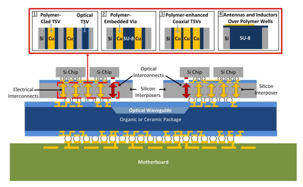
Figure 9: Envisioned silicon interposer based system featuring photodefined (a) polymer-clad TSVs and optical TSVs that can be fabricated simultaneously, (b) polymer-embedded vias, (c) polymer-enhanced coaxial vias, and (d) polymer-enhanced inductors and antennas.
