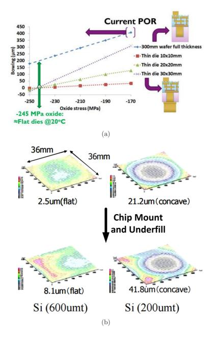
Figure 7: (a) Bow simulation for thinned interposer dice and wafer after TSV, BEOL and bump fabrication, [28] and (b) warpage measurement of silicon interposers from the BGA pad side after chip mount and underfill [35].
