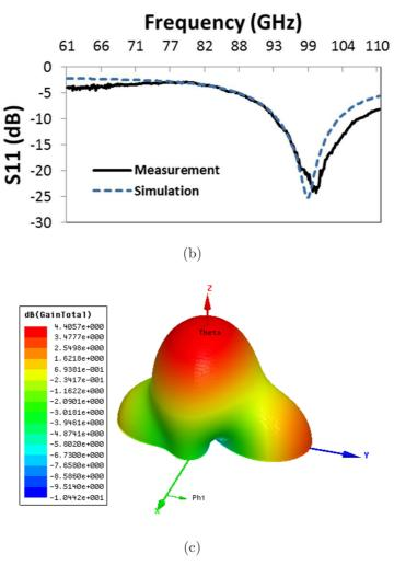
Figure 74: Antenna measurement and simulations: (a) Setup; (b) One-port measurement and simulation; and (c) Radiation pattern simulation at 100 GHz.
