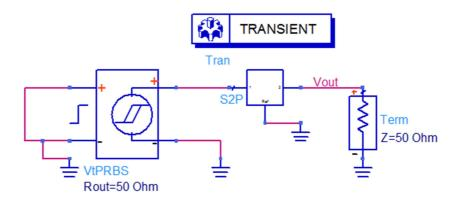
Figure 46: ADS schematic setup for eye diagrams of TSVs.
