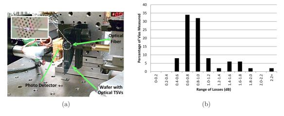
Figure 22: Optical loss measurements for the fabricated optical TSVs: (a) Setup to measure optical loss of the fabricated optical TSVs with an inset image showing optical fiber in contact with an optical TSV and (b) Distribution of the measured optical losses.
