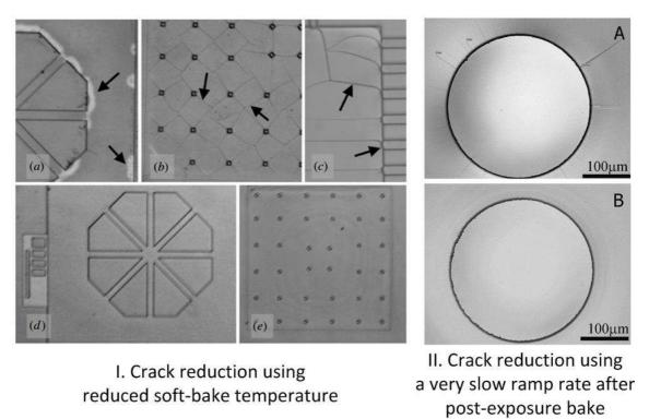
Figure 38: Crack reduction techniques demonstrated in the literature [93, 94]
