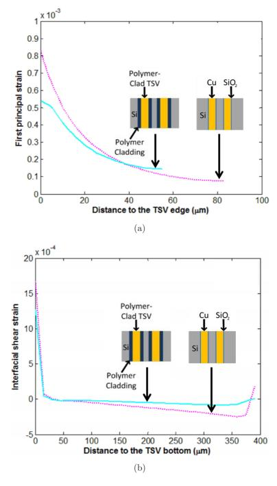
Figure 27: At 150 °C, predicted (a) first principal strain of silicon at the top of TSVs along the path stretching radially away from the liner-silicon interface and (b) interfacial shear strain along copper/liner interface.
