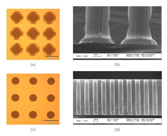
Results of the TSVs Back-to-back Etching with 120, 80, and 25  $\mu m$
