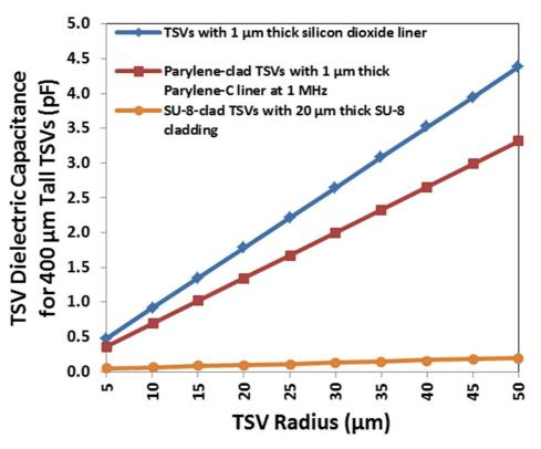
Figure 12: Comparison of TSV dielectric capacitance.
