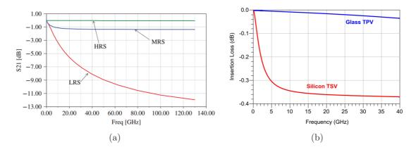
Figure 32: Losses of copper vias (a) in high-resistivity silicon with 75  $\mu$ m diameter and 300  $\mu$ m tall copper vias with a 0.6  $\mu$ m thick silicon dioxide liner [86], and (b) in glass substrate with 15  $\mu$ m diameter and 30  $\mu$ m tall copper vias and in 10 S/m conductivity silicon with 15  $\mu$ m diameter and 50  $\mu$ m tall copper vias with a 0.5  $\mu$ m thick silicon dioxide liner [85].
