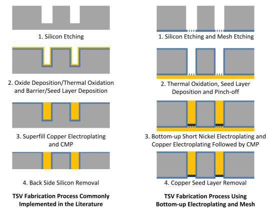
Figure 11: TSV fabrication processes.
