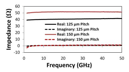
Figure 69: Extracted impedance from the coaxial TSV measurements.
