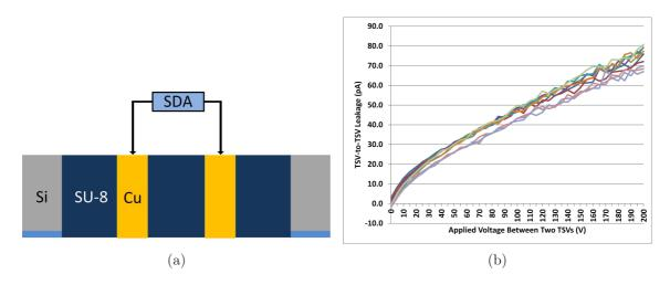
Figure 42: Via-to-via leakage measurement of polymer-embedded vias with 100  $\mu$ m diameter and 270  $\mu$ m height: (a) Schematic of leakage measurement setup and (b) Leakage measurements of 10 pairs of polymer-embedded vias.
