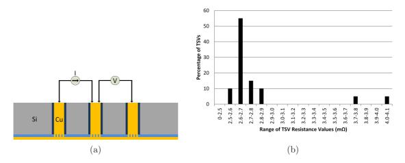
Figure 21: Four-point resistance measurements of the fabricated polymer-clad TSVs: (a) Four-point resistance measurement setup and (b) Distribution of the measured resistance values.
