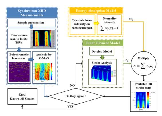
Figure 25: Beam intensity based data averaging method.
