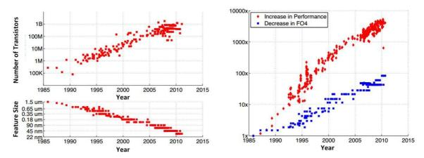
Figure 1: Consistent increase in transistor count, consistent transistor scaling, and improvements in microprocessor performance (normalized to that of a 386) and gate speeds (approximation of the FO4) since the introduction of CMOS microprocessors [4].
