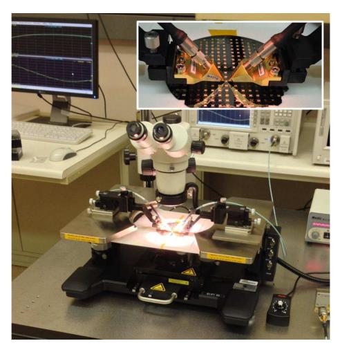
Figure 49: TSV RF measurement setup.
