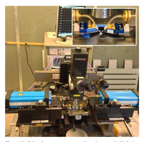
Figure 62: D-band measurement setup for polymer-embedded vias.
