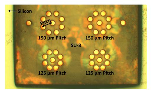
Figure 67: Fabricated coaxial vias for 1-port measurements.
