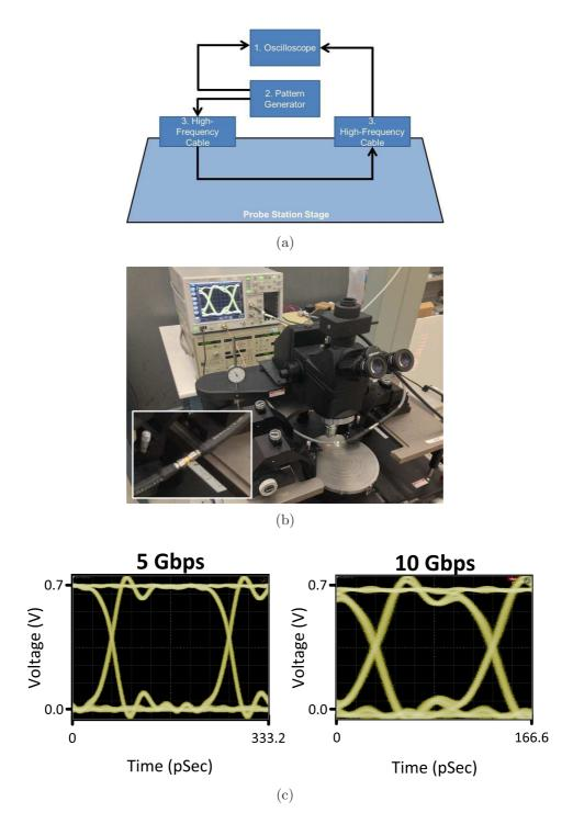
Figure 58: Time-domain loopback characterization (a) schematic, (b) measurement setup, and (c) measurements.
