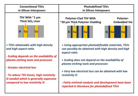
Figure 10: Comparison between conventional and photodefined TSVs for silicon interposers.
