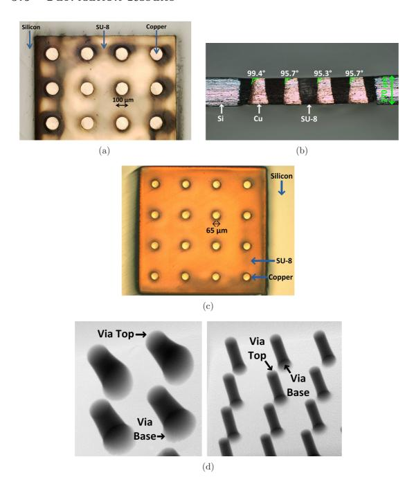
Figure 39: Fabricated 270  $\mu$ m tall polymer-embedded vias on a 250  $\mu$ m pitch: (a) Top view of 100  $\mu$ m diameter TSVs; (b) Cross-section view of the 100  $\mu$ m diameter TSVs; (c) Top view of 65  $\mu$ m diameter TSVs; and (d) X-ray image showing void-free copper electroplating of the 100  $\mu$ m diameter TSVs (left) and the 65  $\mu$ m diameter TSVs (right).
