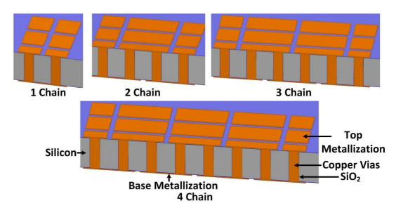
Figure 50: Structures simulated in HFSS for chains of TSVs with silicon dioxide liner.
