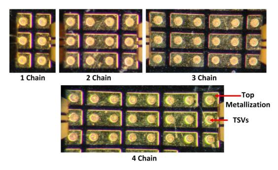
Figure 51: Fabricated chains of TSVs with silicon dioxide liner.
