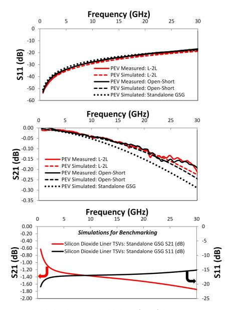
Figure 55: De-embedded polymer-embedded via (PEV) loss using measurements and simulations; TSVs with silicon dioxide liner included for benchmarking.
