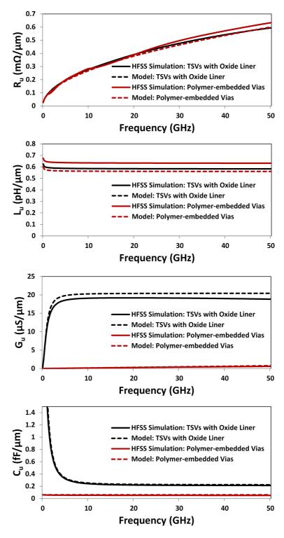
Figure 45: Evaluated per-unit-length TSV RLGC values using circuit models and HFSS simulations.
