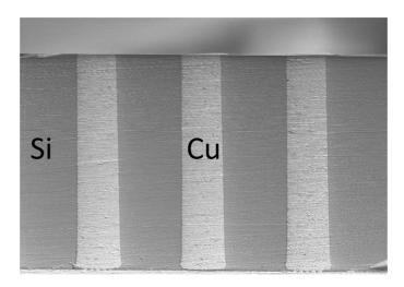
Figure 23: Fabricated 50  $\mu$ m diameter and 300  $\mu$ m tall TSVs with 1  $\mu$ m thick silicon dioxide liner and on a 150  $\mu$ m pitch.
