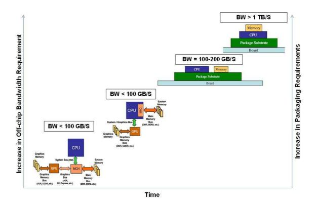
Figure 3: Increase in off-chip bandwidth and demand for innovative interconnection and packaging technologies. Images in the plot are from L. Polka et al. [8].
